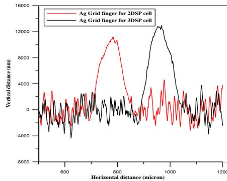
**Figure 1.** Telestep Profiles of Ag-grid Fingers of 2DSP and 3DSP cells
