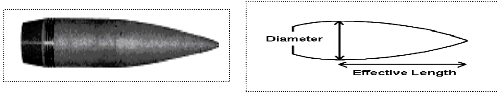
Figure 2: Schematic of Artillery Projectile and its Effective Length
